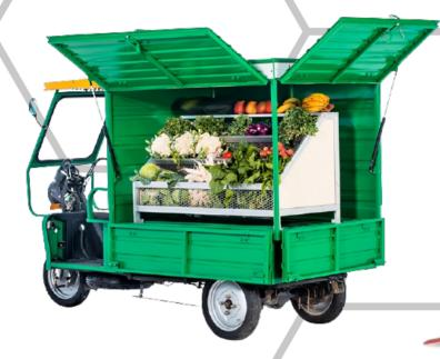
ICAT Approved And RTO Approved Wind Shield And Wipers Headlights And All Side Indicators Hydraulic/manual Tipping Facility Front And Rear Drum Breaks 43 Mm Front Shockers Leaf Spring For Rear Suspension 180 Mm Ground Clearance Single Speed, 25 Km Max Speed
